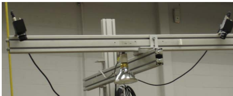
Figure 2: Camera setup for 3D binocular stereo vision
