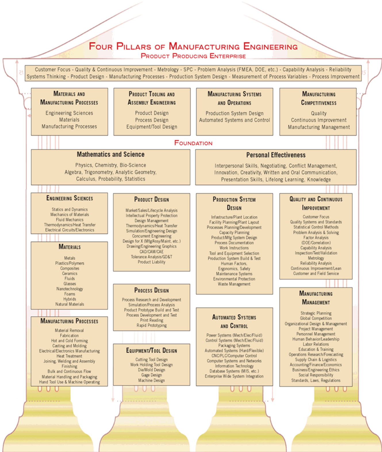
Figure 1. The SME Four Pillars of manufacturing engineering. (Mott et al., 2012; Mott et al., 2013; SME, n.d.). Reprinted with permission.
