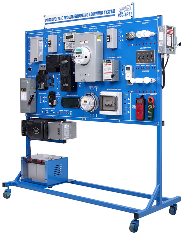
Figure 4. Solar PV troubleshooting. Reprinted with permission.
