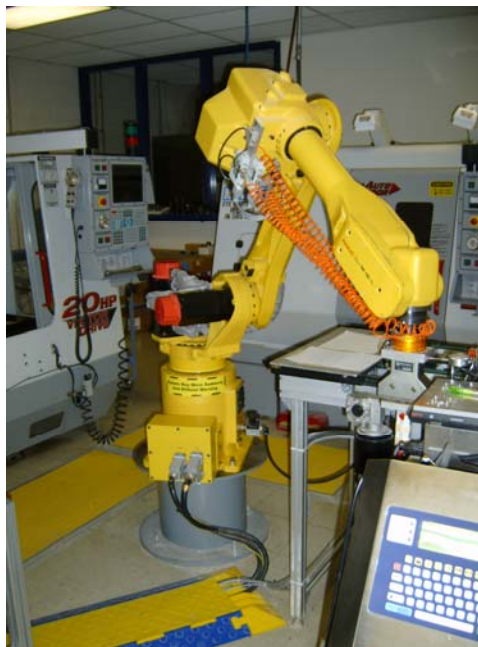
Figure 1. The Fanuc M16iL 6-axis industrial robot used in this study.
