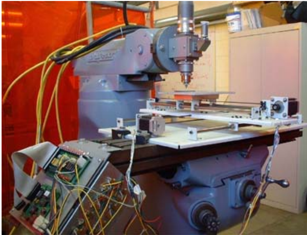
Fig. # 12: The X-Y Table System in Laser Welding Applications
