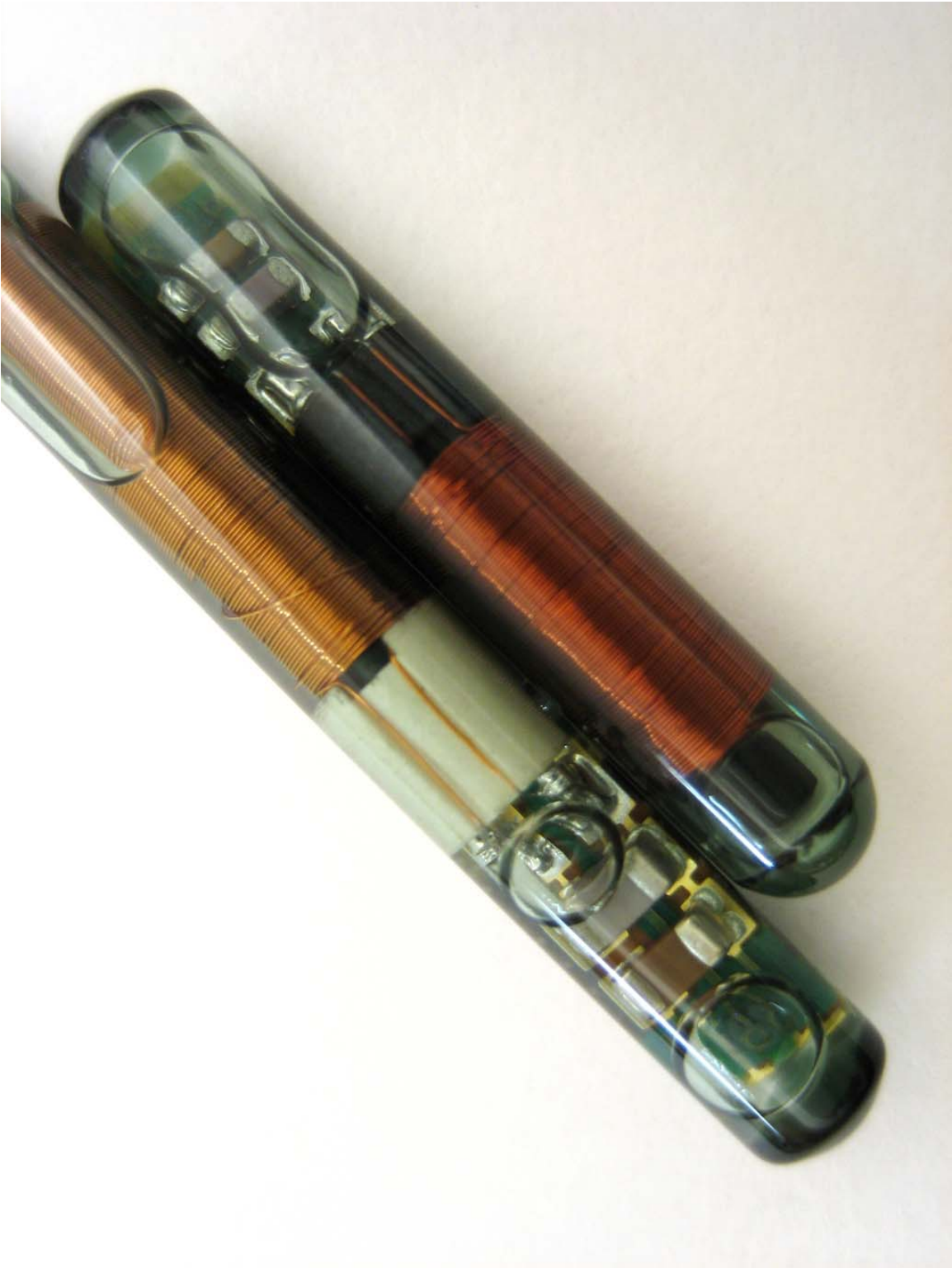
FIGURE 4. RFID tags in the LF range suitable to be implanted in animals. The length of these tags is 1" and 1.5". In this close up it is easy to observe the coils that make the antennas for these tags.
