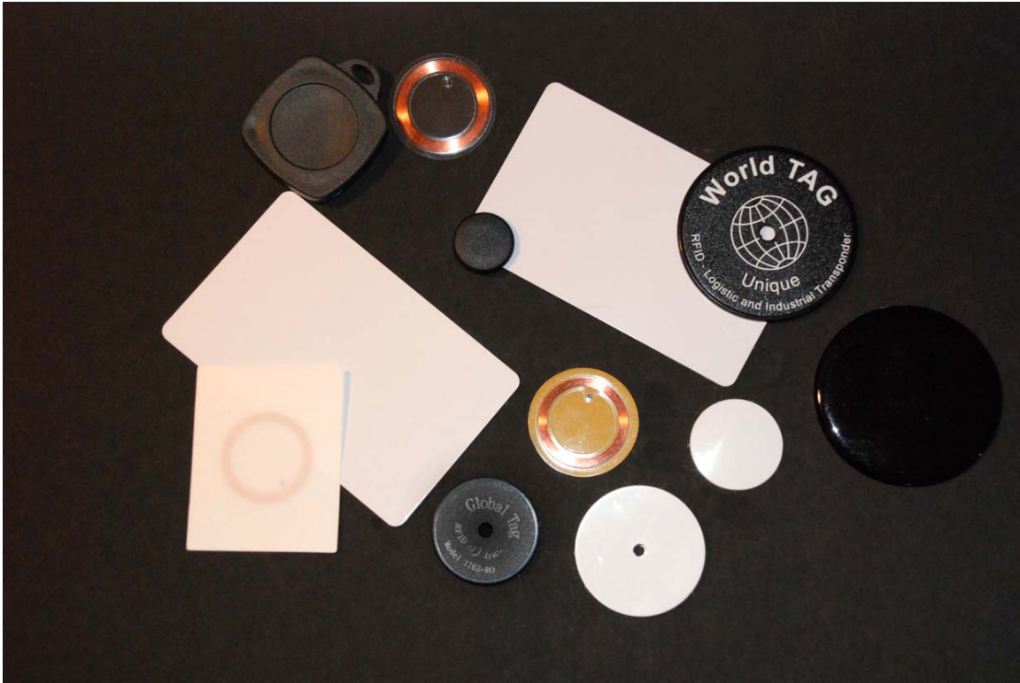
FIGURE 3. Several tags that operate in the LF range. These tags are available in different shapes and sizes, but because of the requirements in the 125 kHz to 140 kHz frequency range, all the tags require considerable wire length for to make their antennas efficient. The length of cable required can be seen in the transparent tags. In these same tags, it is also possible to see the chip that is connected to the antenna.
