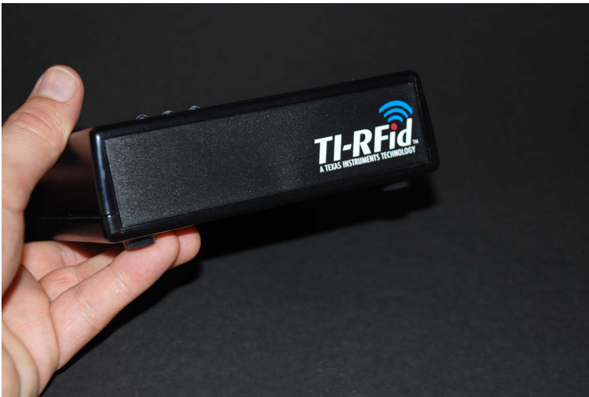
FIGURE 10. Evaluation RFID module from Texas Instruments. These modules can operate at LF and HF frequencies.
