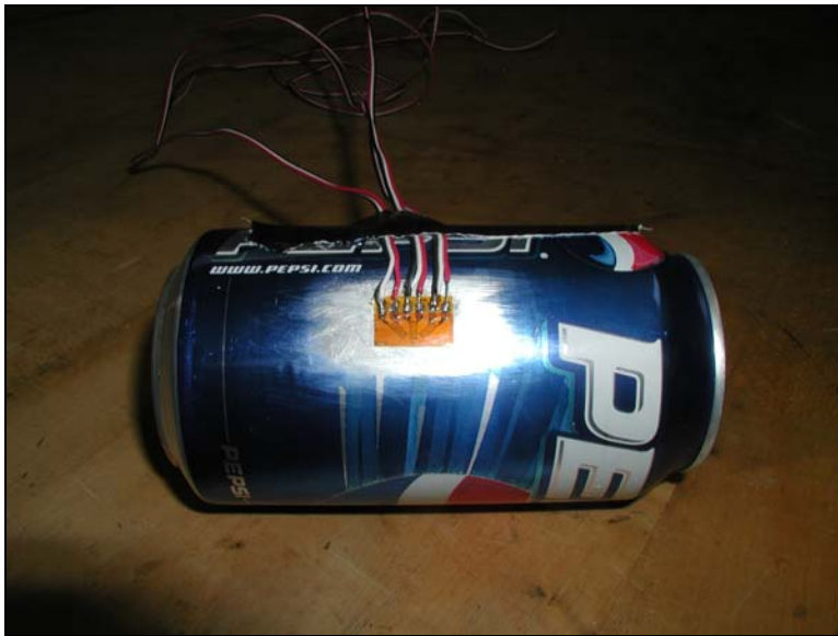
Figure 2 – Rosette strain gage mounted on a soda can with an arbitrary alignment. Principal strains must be calculated to determine the hoop and longitudinal strains.
