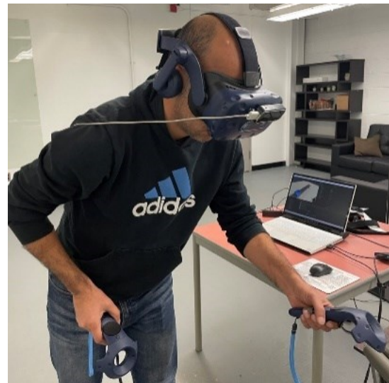
(a) Subject wearing HTC Vive immersive head-mounted display, two controllers, and Leap Motion.
