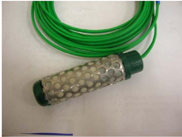
Figure 9. Watermark Soil Moisture Sensor
