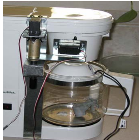
Figure 9. Assembled coffee pot showing Final Drop Float level sensor and wiring through the lid
