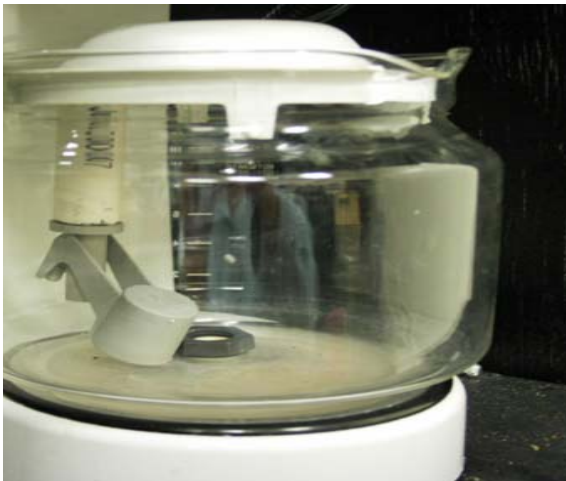
Figure 8. Drop Float level sensor
