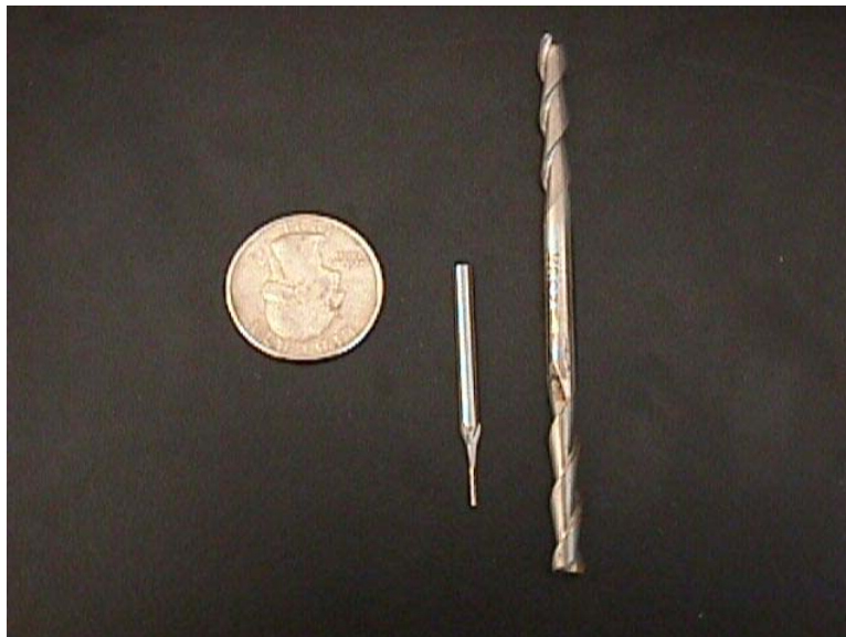
Figure 8 Comparison of 0.250" and 0.032" End Mill
