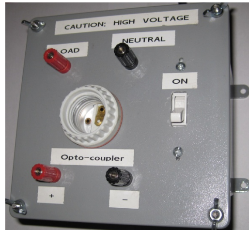
Figure 2: New thyristor fixture design, top-right view
