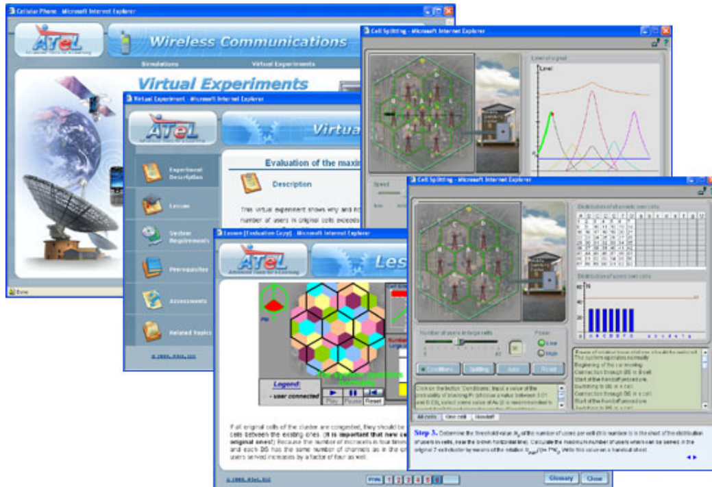
Figure 3. Screenshots of the virtual lab that enable students to explore the number of mobile phone users that can be served by a wireless local area network (WLAN) and the Cell Splitting procedure. While studying the procedure, students can vary blocking conditions, number of subscribers in large cells, determine the threshold, split the cells and assign the channels to the microcells, and investigate handoff process in a WLAN of different configurations. The simulation runs with a detailed step-by-step instruction for the student on how to perform the experiment. Students are able to collect virtual data and record them on the provided worksheet. An interactive lesson incorporated in the lab (bottom left) facilitates “just-in-time” learning of underlying scientific or engineering principles. Each virtual experiment includes an associated test.
