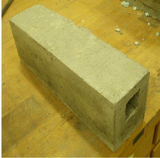
Figure 3. One of Several Hollow Beams Cast at GSU
