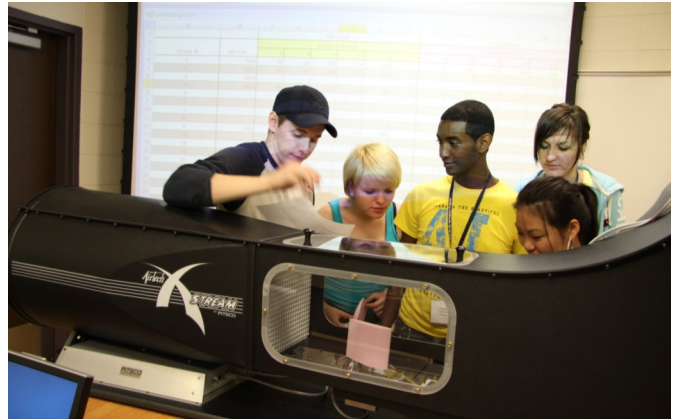
Figure 6. Undergraduate Assistant Helps GFA Students Test Their Airfoil Designs
