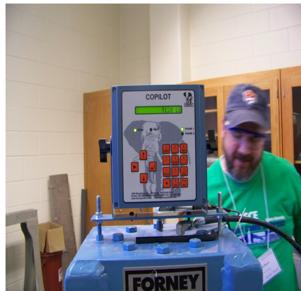
Figure 5. Display of Failure Load (9,120 lb.) for GSU Team's Beam at the Competition
