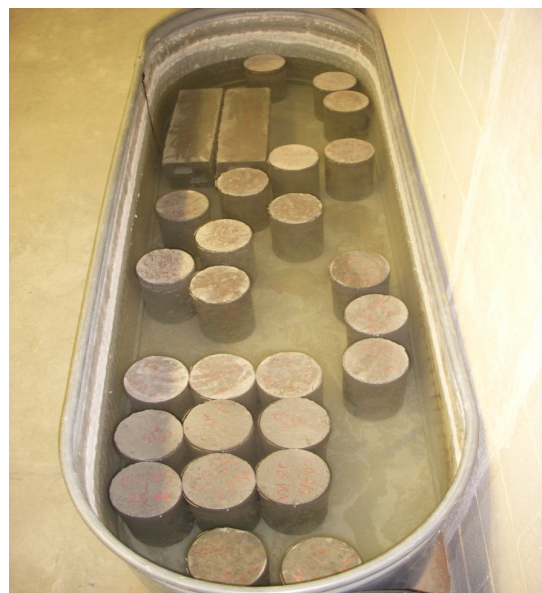
Figure 2. Beam and Cylinder Specimens Being Cured at GSU
