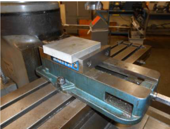
Figure 3. Clamping Position to Machine First Y Axis
