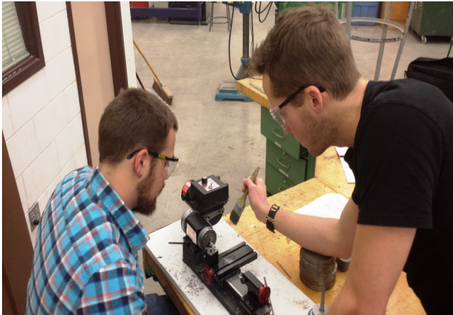
Figure 14. Technology Students Machining the Center Punch in Stage 2
