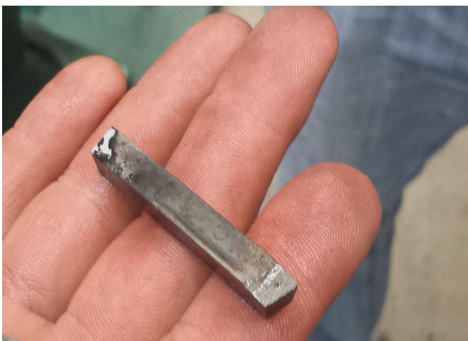
Figure 12. Lathe Cutter Produced in Stage 2
