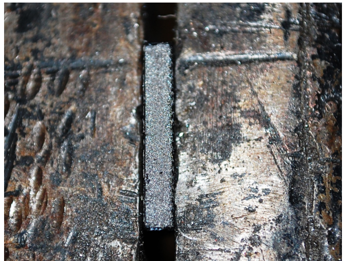
Figure 11. Example of Coarse Grain Structure in a Test Strip from Stage 1
