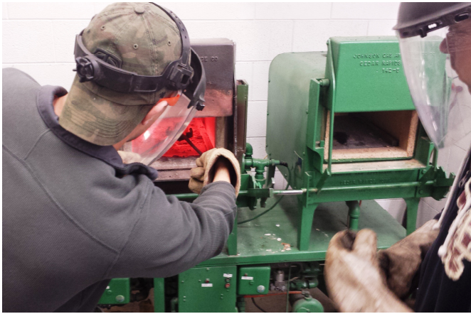
Figure 5. Technology Students Heat Treating a Spring in Stage 1
