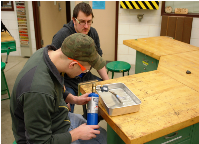
Figure 9. Technology Student Differentially Tempering Steel Strips in Stage 1
