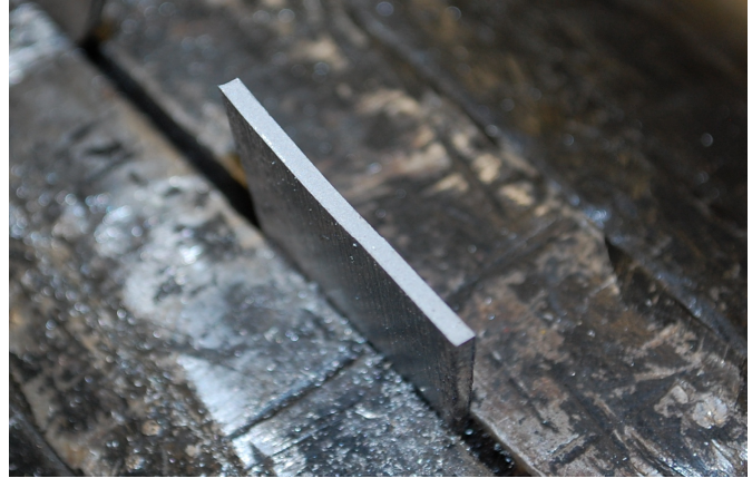
Figure 7. Observing the Fine Grain Structure in the Steel Test Strip from Stage 1
