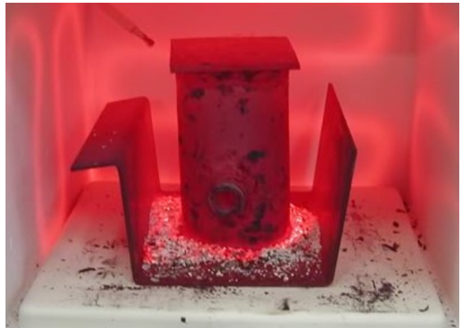
Figure 3. Crucible for Carburizing Parts in Stage 1
