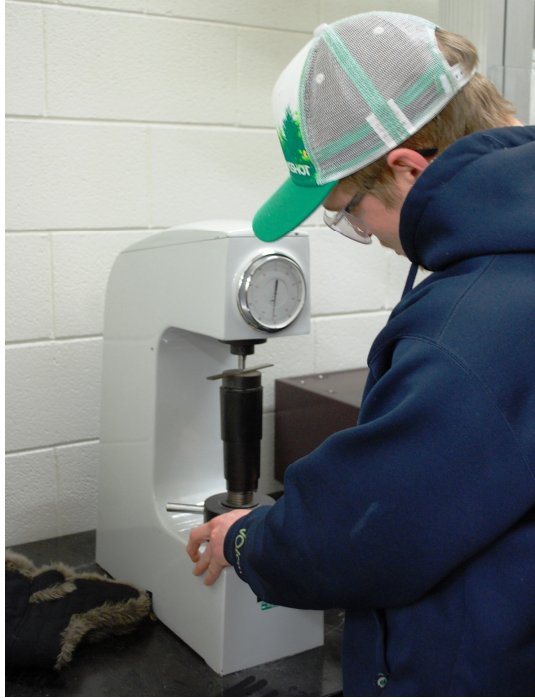
Figure 17. Student Verifying Rockwell Hardness after Heat Treatment
