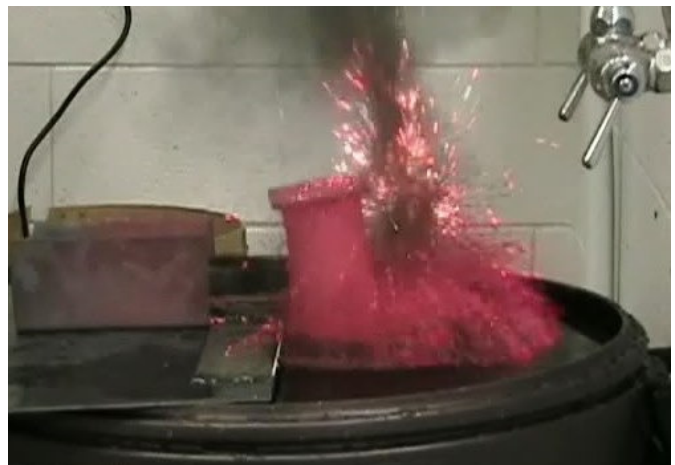
Figure 4. Sparks Fly as the Lathe Cutter is Quenched in Stage 2
