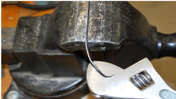
Figure 18. Testing a Completed Spring
