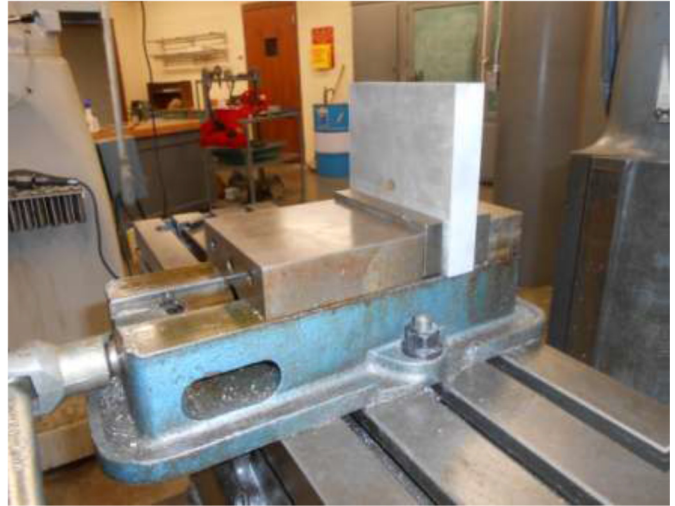
Figure 4. Processing Final Y Axis with Aluminum Block Placed Vertically in Vise
