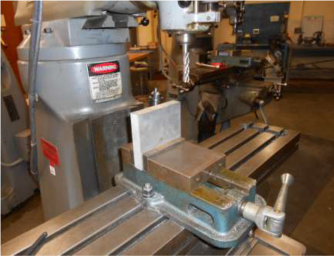
Figure 2. Aluminum Block with Factory Edge Against the Base of Vise
