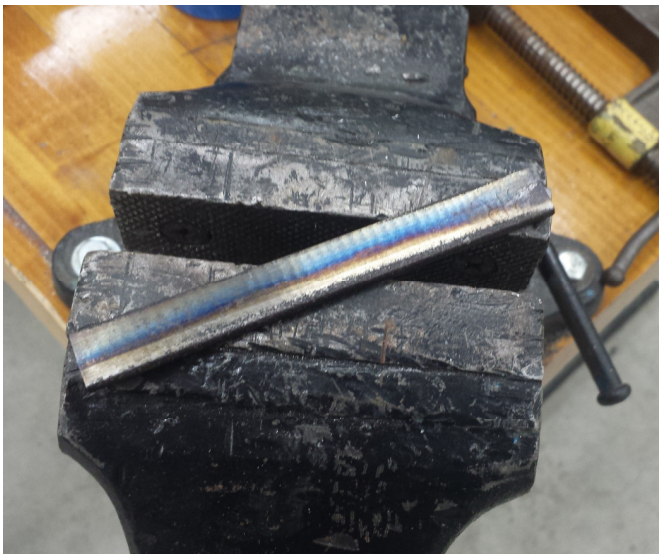
Figure 10. Differentially Heat-treated Test Bar, as Produced in Stage 1
