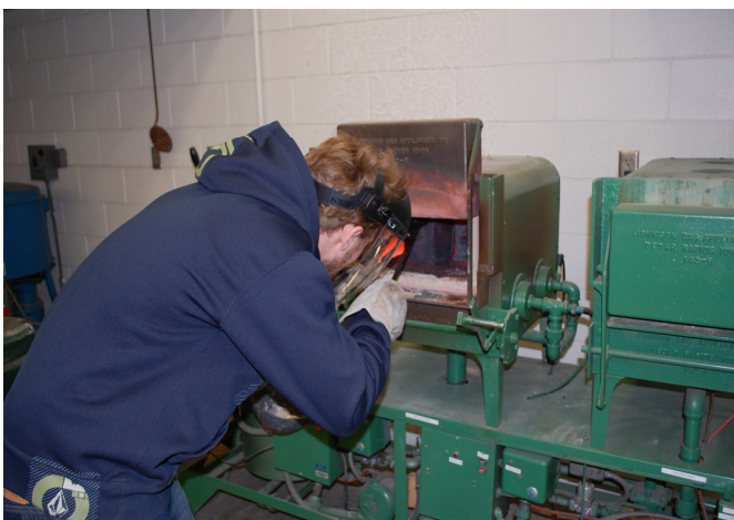
Figure 6. Technology Student Placing Crucible Containing the Lathe Cutter in the Furnace for Carburizing in Stage 1
