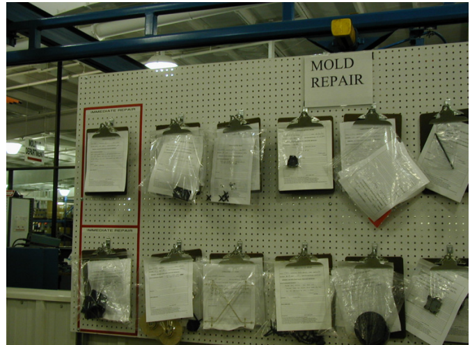
Figure 2. FIFO Lanes Used to Control Work Sequence
