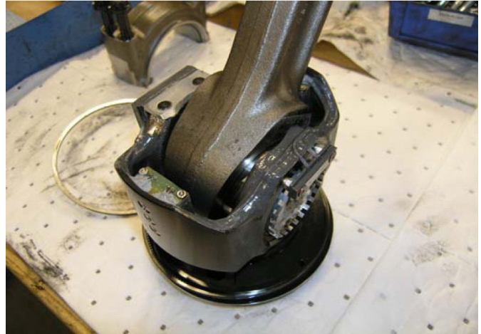
Figure 1. Piston and Rod Combination Outfitted with Pin Temperature and Rotation Sensors [12]
