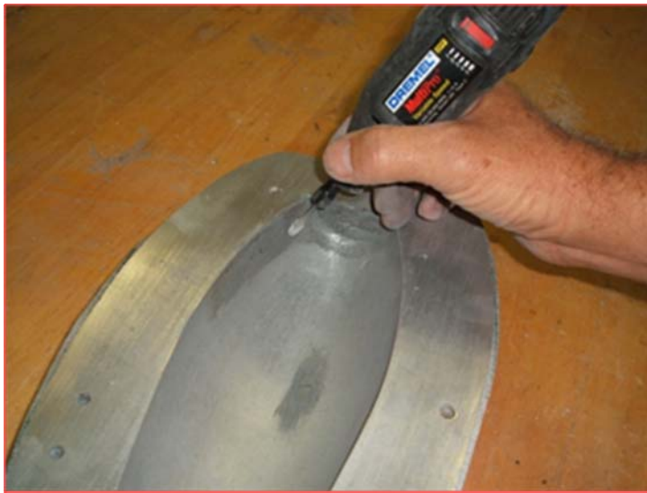
Fig. 28 Removing Filler – Smoothing Mold Surface
