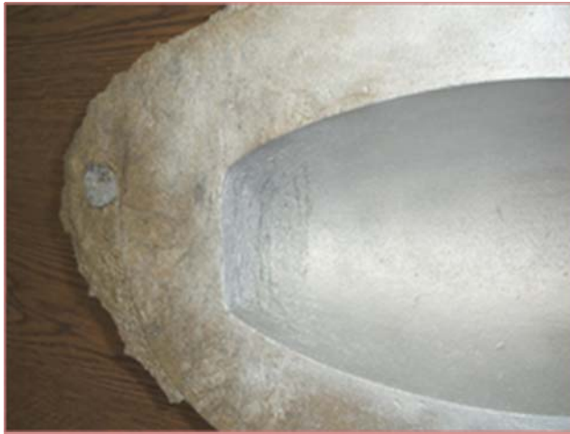
Fig. 26 Casting Defect - Porosity
