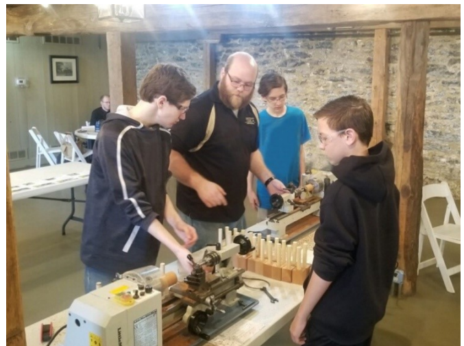
Figure 4. High school students working with a Millersville University graduate student to turn wood ball and cup toys on a 7"x16" bench-top metal lathe produced by Little Machine Shop.
