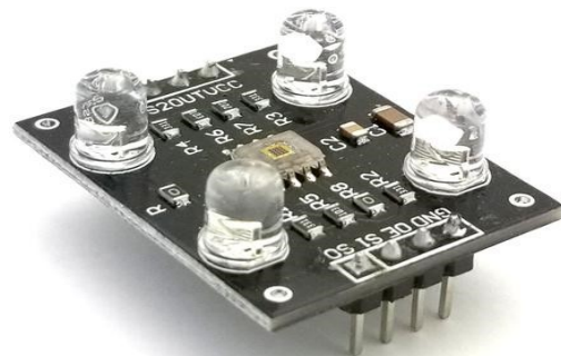
Figure 1. TCS3200, a common Arduino color sensor.
