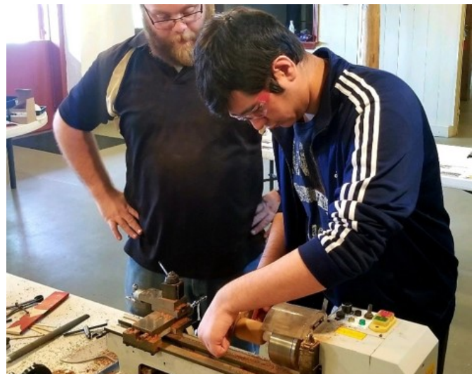
Figure 6. High school students working with a graduate student to sand the ball and cup toys on a bench-top metal lathe.
