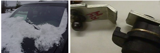
Figure 10. Windshield Wiper under Snow Load Breaking a Rocker Arm
