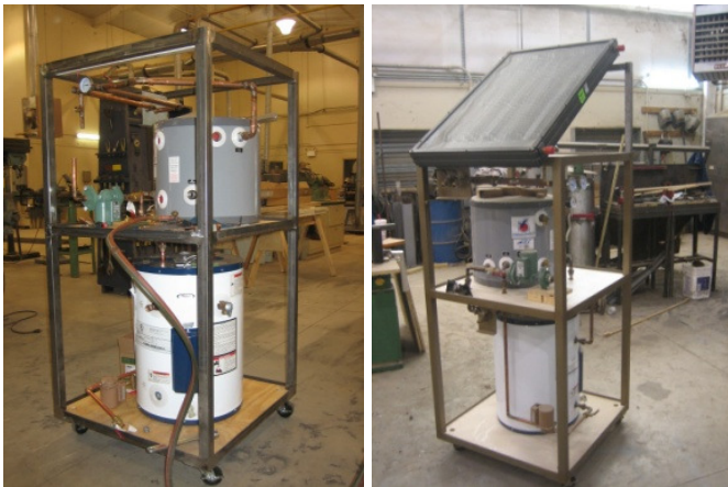
Figure 3. Passive Solar Water Heating System
