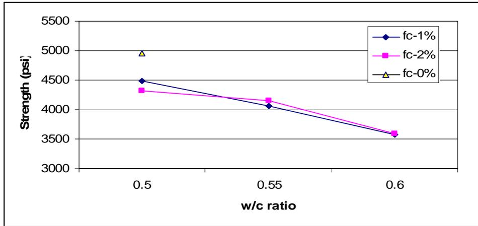
Figure 4: Compressive strength versus w/c ratio
