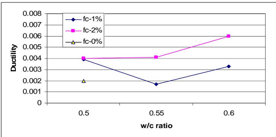
Figure 6: Ductility versus w/c ratio
