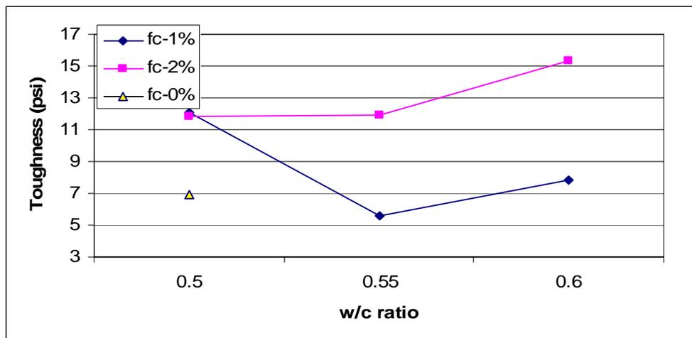
**Figure 8: Toughness versus w/c ratio**
