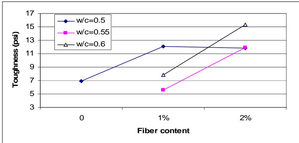
**Figure 9: Toughness versus fiber content**
