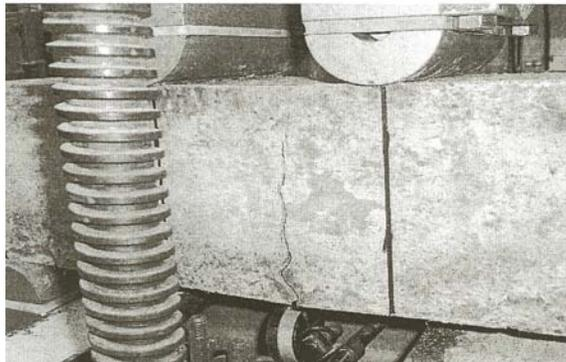
**Figure 3: Beam failure in the MOR test**
