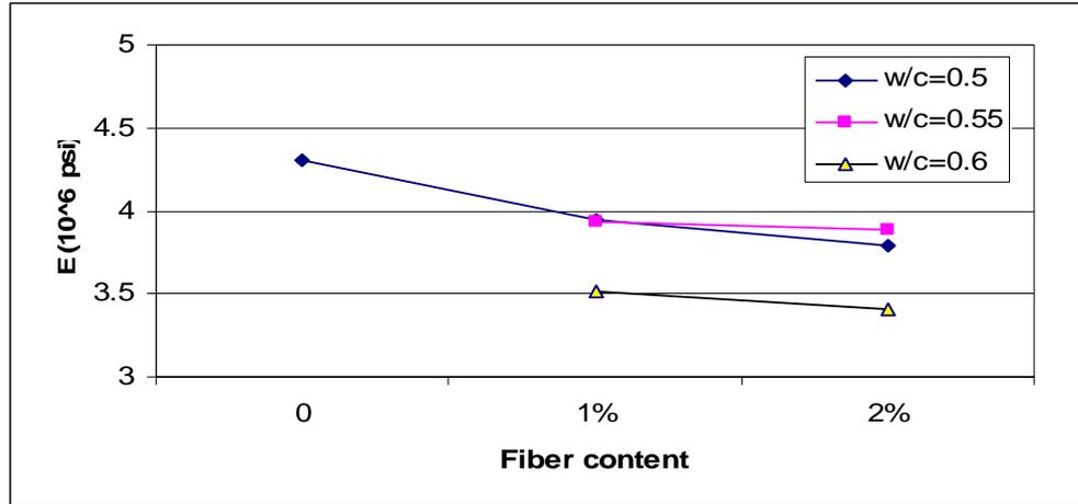
**Figure 11: Modulus of elasticity versus fiber content**
