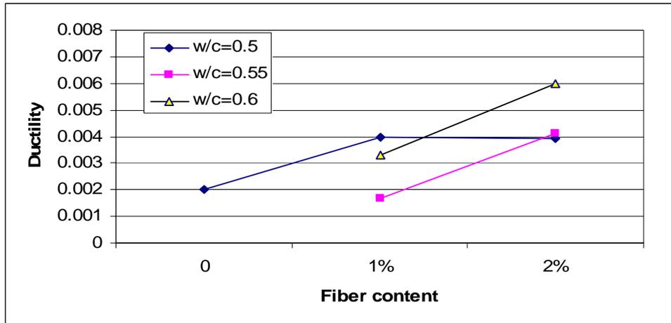
**Figure 7: Ductility versus fiber content**
