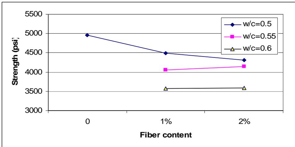
Figure 5: Compressive strength versus fiber content
