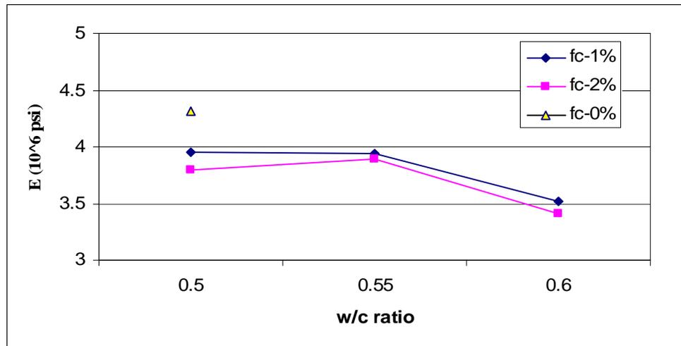
**Figure 10: Modulus of elasticity versus w/c ratio**
