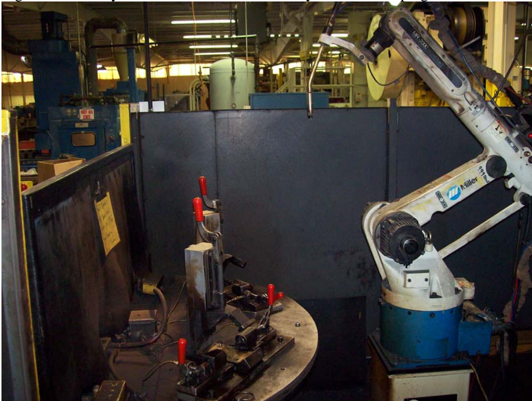
Figure 1: Turn Style Robot Welder used at Duffy Tool & Stamping L.L. C.
