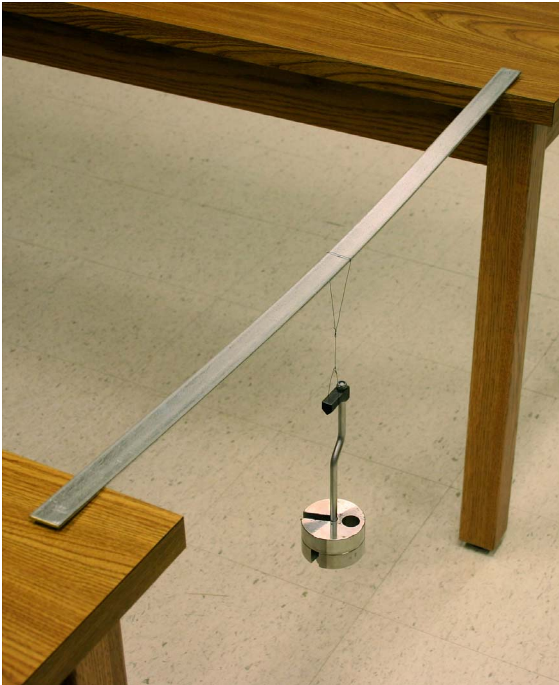
Fig. 1: Weights hang from a beam supported by two classroom tables. Flatstock has a lower tendency to roll than round rods.
